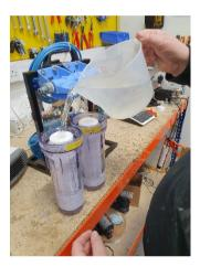
completely fill the jars with water with filters present.
