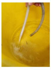
Operate the pump switch and ensure water is flowing at the waste out hose
