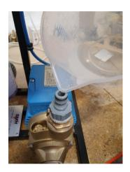
Fill the pump motor housing with water by pouring water into the waste out tap connector.
