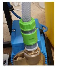
Ensure the tap connector has a solid seal. Any air leaks will cause failure to transfer water.
